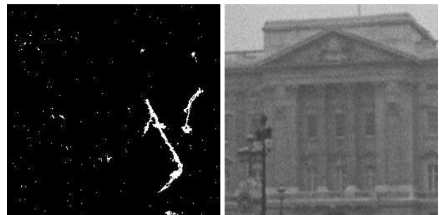
Figure 7: Detection (left) and removal (right) of impulsive defects on frame 30 of the Building sequence
