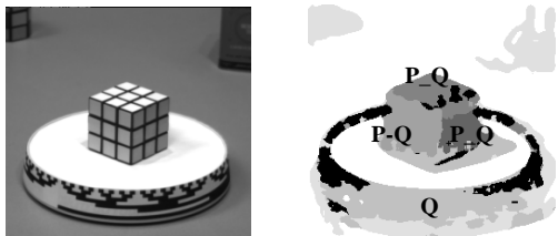
Figure 4: Result of our Motion Segmentation. Q indicates that the selected model is Quadratic while P-Q indicates that the chosen model is partial quadratic (based on the GMDL criteria).
